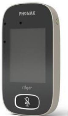
The microphone, worn close to the teacher's mouth, picks up the teacher's voice, and the sound is then transmitted to the child's receiver. This enables the teacher's voice to be received directly into the hearing aid or processor, wherever they are in the room, giving a more consistent and much improved signal to noise ratio.
